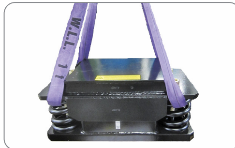
Fig. 4: Lifting of spring element with sling
