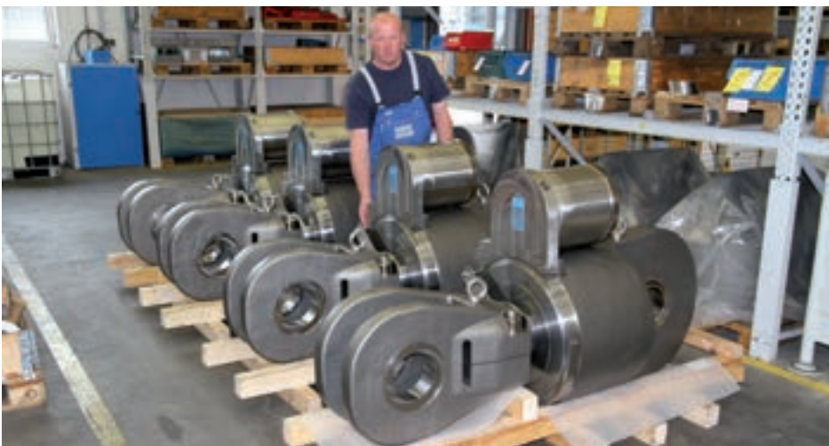
Final inspection of snubbers type 31
