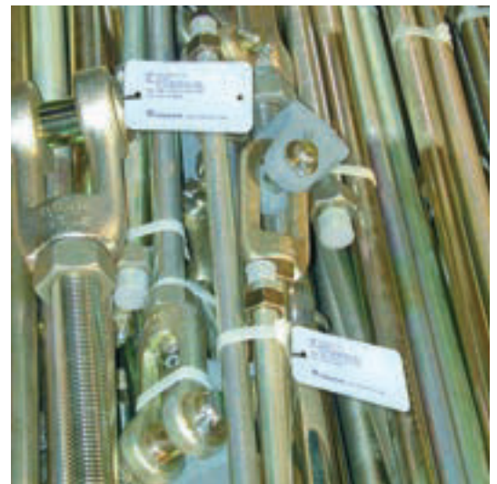
Load chains, pre-assembled, bundled and marked
