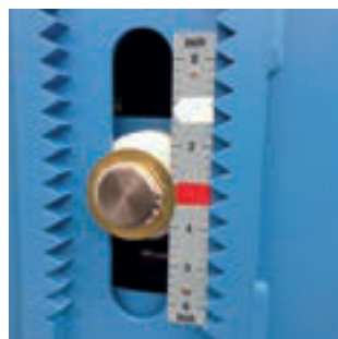
Travel scale with cold/hot marking
