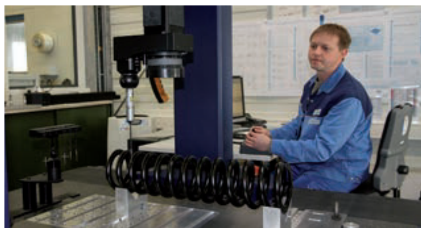
Spring testing at material reception
