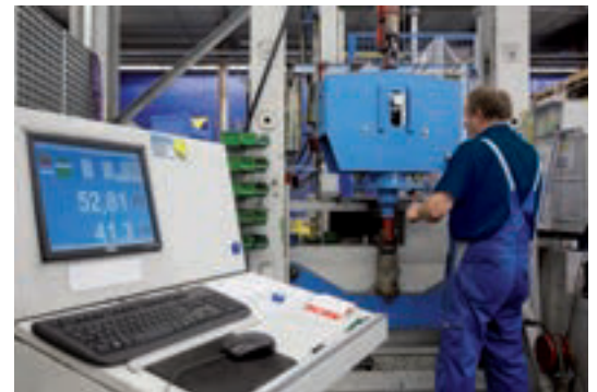
Acceptance testing of a constant hanger
