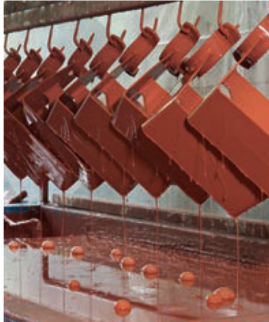
Cataphoretic immersion priming
