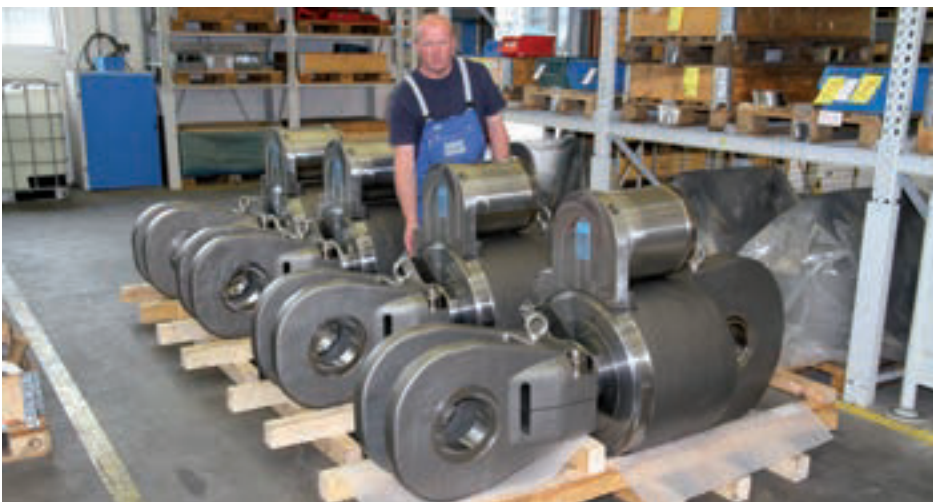
Final inspection of snubbers type 31
