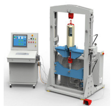
Testing a spring hanger on a LISEGA 120kN test bench
