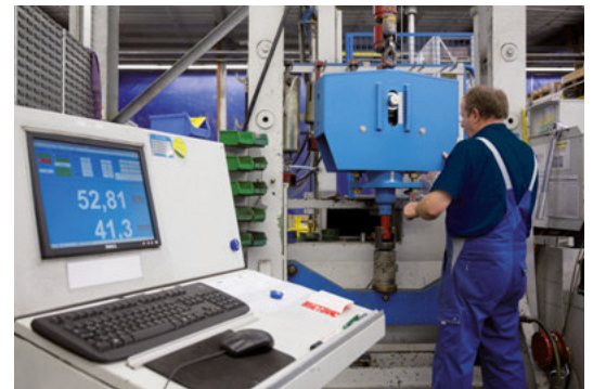
Acceptance testing of a constant hanger
