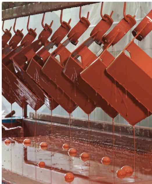
Cataphoretic immersion priming
