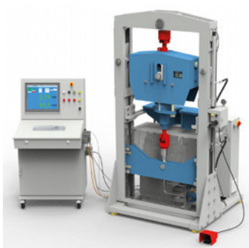
Testing a constant hanger on a LISEGA 120kN test bench
