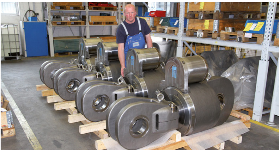
Final inspection of snubbers type 31
