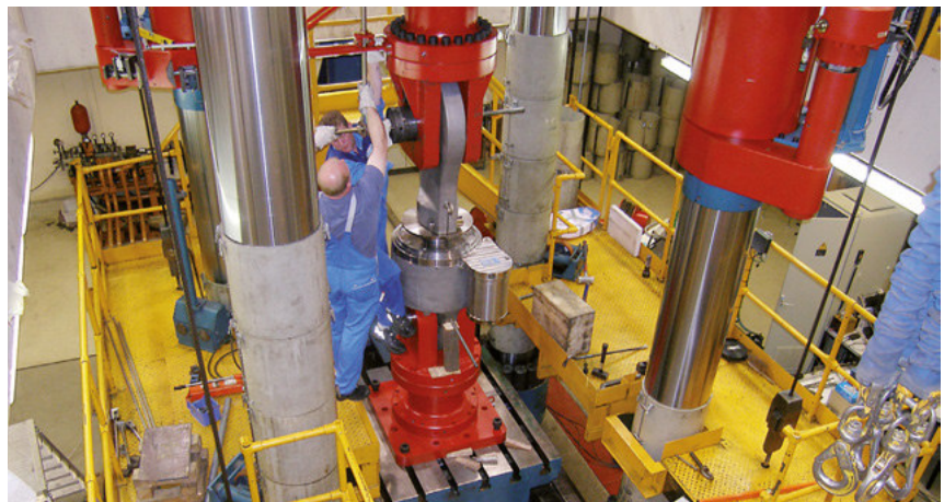
Special testing of snubbers type 31. Test load up to 8600kN.
