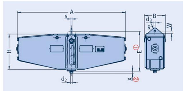
① Dimension E for uppermost blocking position, in other blocking positions E lengthens accordingly.
