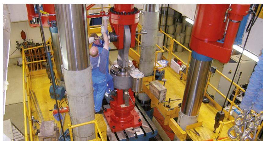
*Special testing of snubbers type 31. Test load up to 8600kN.*
