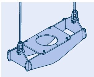
Riser clamp type 46 with connection components
