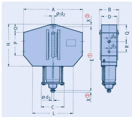
① Dimension E for uppermost blocking position, in other blocking positions E lengthens accordingly.
