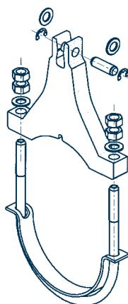
For installation the pre-assembled U-bolts must be removed. The upper part, fitted with a lug recess, is seated on the shear lug. The U-bolt is inserted from the opposite side together with the shim plate and at first only loosely screwed. The position of the clamp is to be checked again for proper alignment. The bolts can then be tightened and locked.
