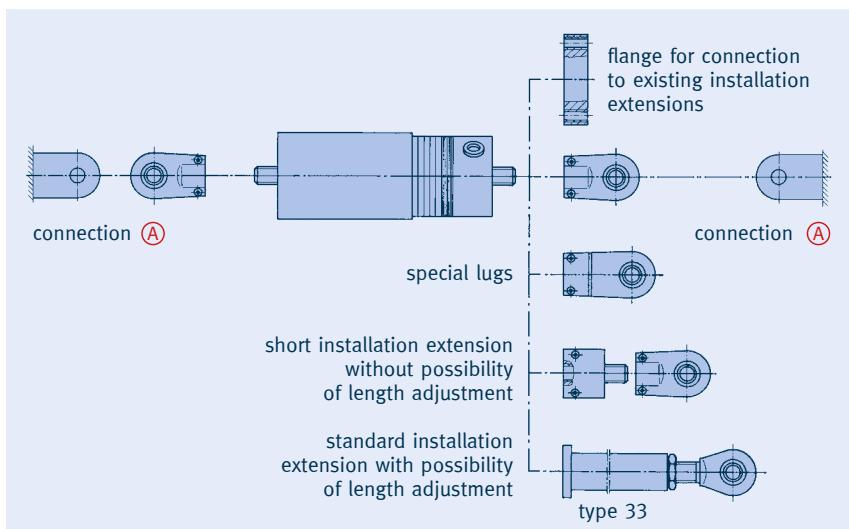
(A) Connection possibilities: See pin diameters of weld-on brackets type 35 or dynamic clamps in product group 3.
