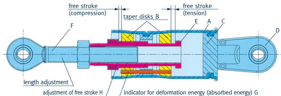
The design consists of an austenitic tubular casing (A) with defined size, into which taper disks (B) with defined force have been pressed. The tube is sealed with a fixed base (C) fitted with a connecting lug (D). The force transmission over the whole unit is made via the stops (E) and the push rod (F).
