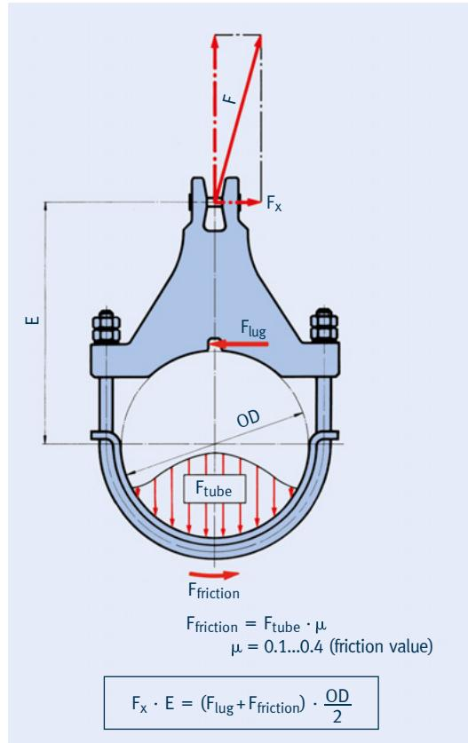
To secure dynamic clamps type 36/37 against misalignment due to compressive stress and off-axis load applications, LISEGA offers standardized shear lugs.
