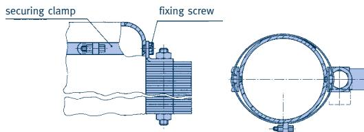
If the original blocking devices have been misplaced and the spring needs to be blocked, e.g. at revisions, they can be supplied by LISEGA at short notice.
