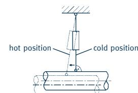
Rods vertical in installation condition
