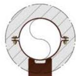
Threaded parts and boltings of the straps, plates, U-bolts and clamps of the pipe-surrounding components must, for increased corrosion protection and a working temperature over 350°C, be located within the insulation in accordance with the installation instructions.
