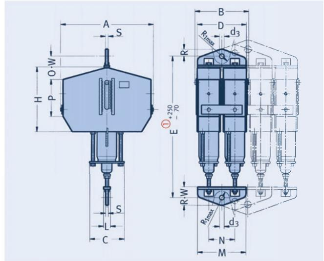
① Dimension E for uppermost blocking position, in other blocking positions E changes accordingly.
