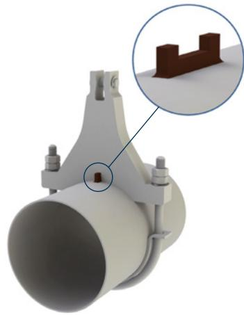
Force distribution in a dynamic clamp with shear lug
