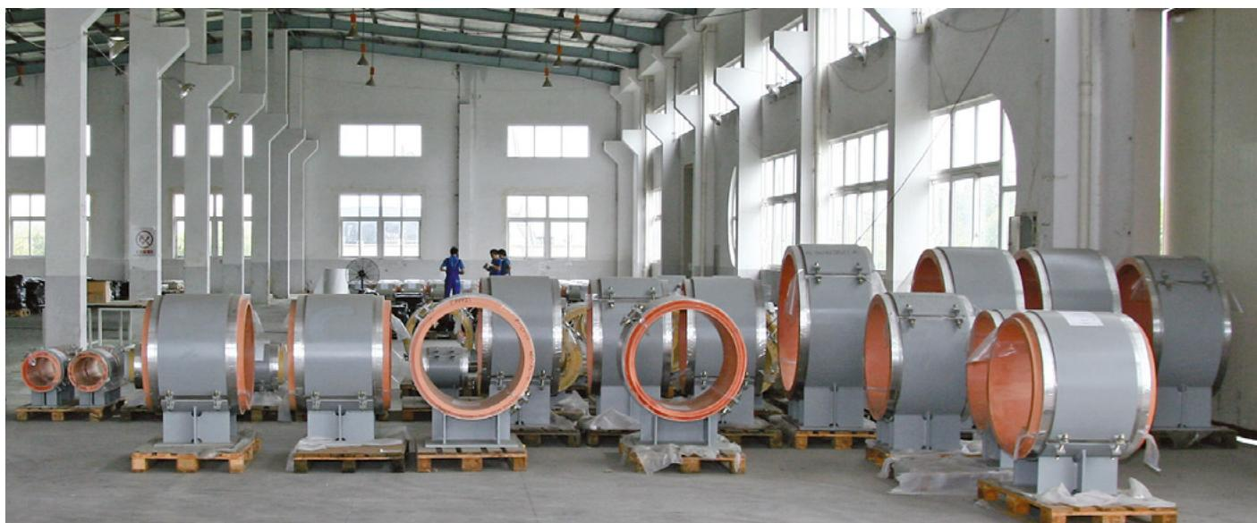
*Preassembled insulated pipe supports*
