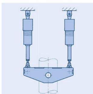
Type 34 with snubbers type 30 and twist restraints
