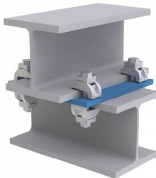
The safe connection of beam profiles to each other is produced very easily with an inlay plate and 8 LISEGA beam adapters. The load-bearing capacity of a cross-connection can be found in the table below.
