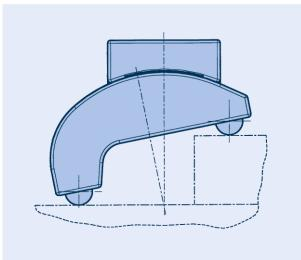
*Typical utilization of beam clamps
