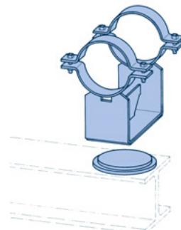
The installation height of the clamp base increases by approximately 3mm.
