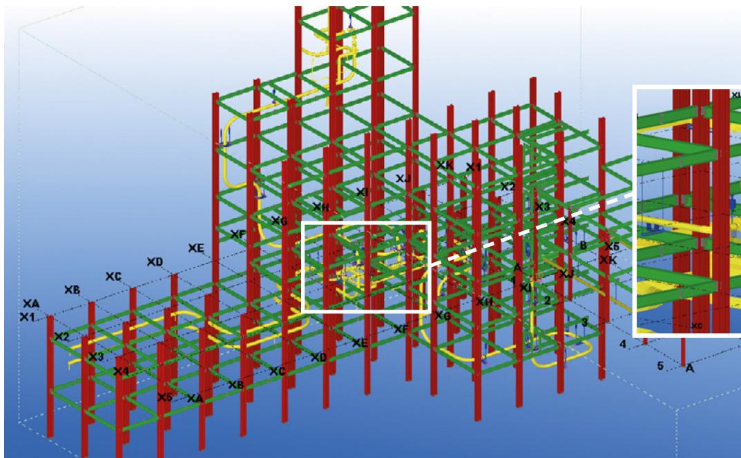
Primary steelwork and pipe systems with supports as reference in TEKLA®
