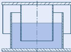
Construction of the LISEGА viscoelastic damper
