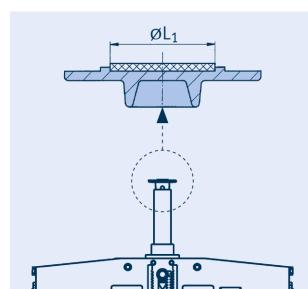
Load plate with integrated slide plate. This must be considered in the selection of clamp bases.
