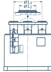
When using slide plates the sliding surfaces of the mating component should be fitted with stainless steel plating. This is indicated by the suffix "SP" in the type designation (e.g., clamp base type 49 97 14-SP).
