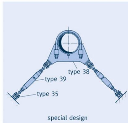
5. When arranging components, **sufficient lateral freedom of movement** must be ensured so that no jamming occurs at the connections.
