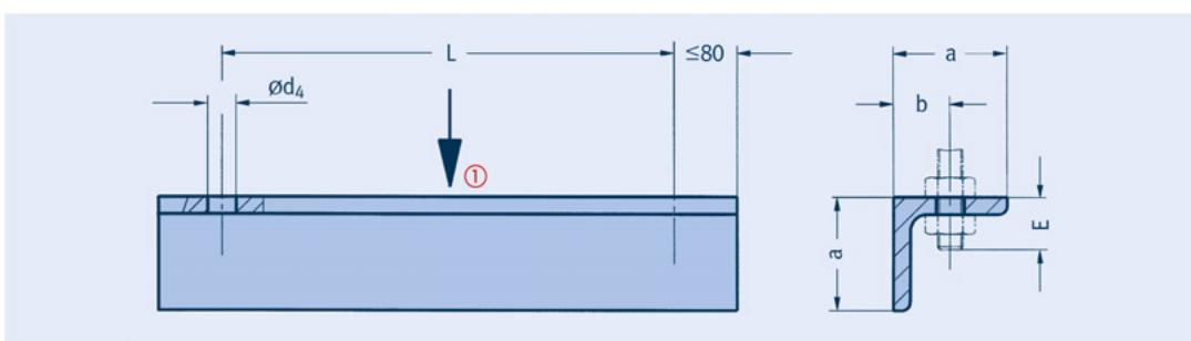
**Trapezes for the use of lower loads at temperatures  $\leq 80^{\circ}\text{C}$**
