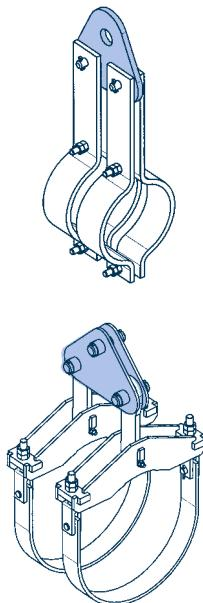
*By coupling two pipe clamps with connection plates type 77 the loads can be doubled. A selection can be found on page 4.67.*
