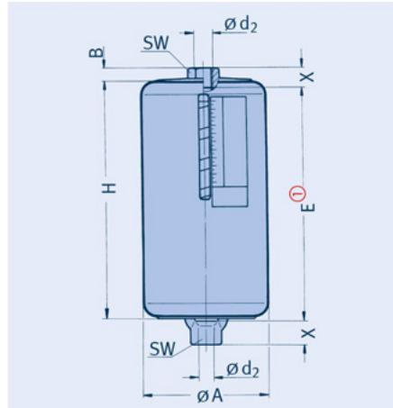
① Dimension 'E' increases on loading by the corresponding spring travel (see load table on page 2.5).
