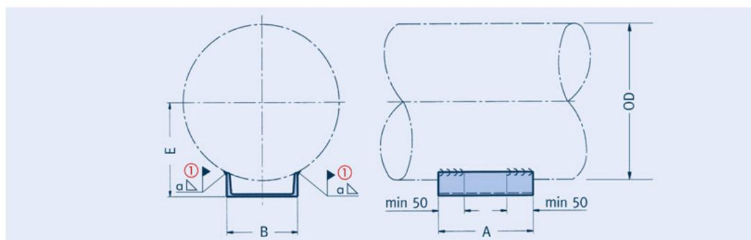
① Weld seam on site – for specified weld seam thickness and permissible load, the weld seam stress is smaller than  $50\text{N/mm}^2$ .
