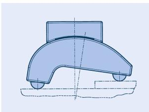
The hardened support segments have a circular groove profile that is pressed into the contact surface on tightening. This way, a **form-fit contact is produced which ensures that no shifting in any direction takes place.**
