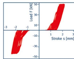
*Measured force/travel path with oscillating loads > nominal load*
