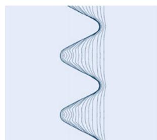
Fiber flow of rolled thread
