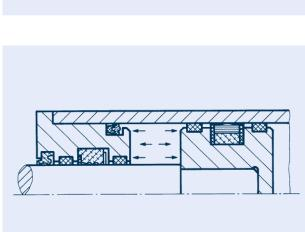
The most important requirement for a long-lasting sealing effect is the choice of the correct sealing material. The crucial factor thereby is the seal's restitution behavior ('shape memory') or compression set, providing the lowest possible stress relaxation.
