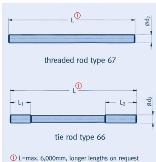
Connecting rods from M56x4 can be supplied as threaded rods type 67 or as tie rods type 66 with individual rolled thread lengths.
