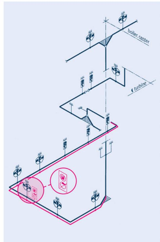
Through use of the hydraulic servo support the pipe system can now be repositioned to the specified elevation.
