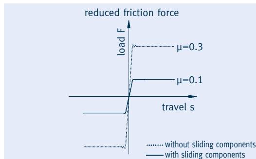
Reduction in reaction forces in the piping system by the use of slide plates.
