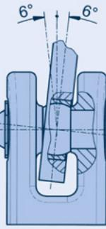
The ball bushing joints for the
