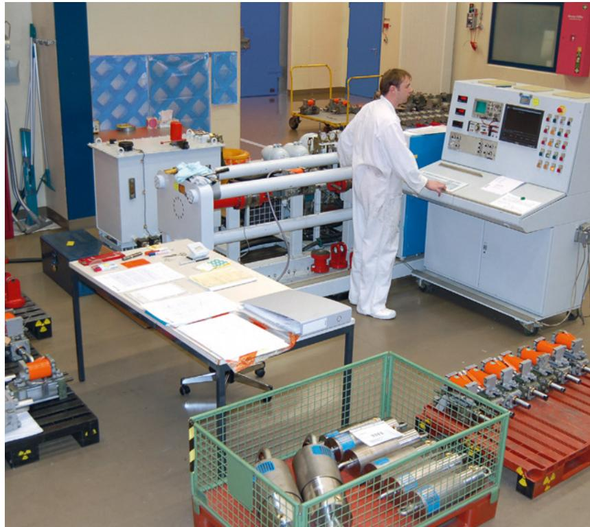
*Testing snubbers of different makes at the plant using a mobile LISEGА test bench.*
