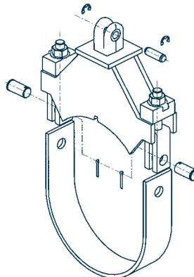
The position of the clamp must be checked once again for proper alignment. The bolts can then be firmly tightened. To avoid unintentional loosening the hexagon nuts on the bolts must be locked with tab washers.
