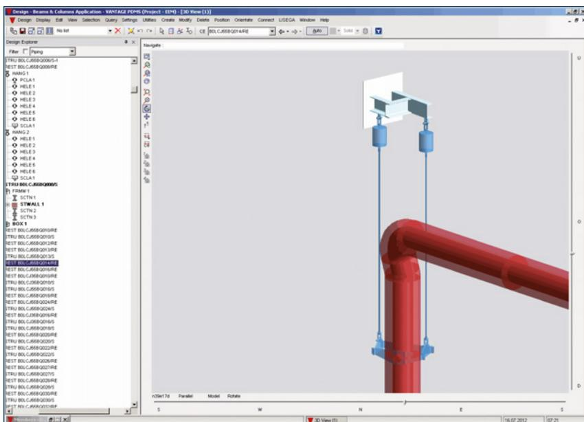
**Step 4:** Integration of the LICAD® support into the 3D model with collision analysis and integration of secondary steelwork
