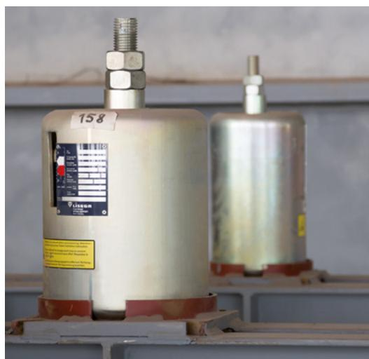
As standard practice, the permissible force deviation between cold position (blocking position) and hot position should not exceed 25 % in relation to the hot load.
