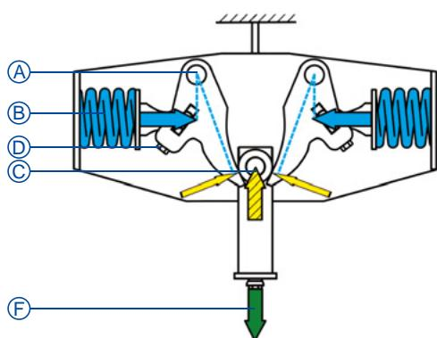
Sinus-shaped load deviations from the lever movement in the form of an arc are balanced by correspondingly machined cam profiles. This way the load distribution is held constant with mathematical accuracy in every position.
