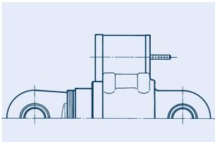
The snubbers form a closed hydraulic system **without external bolted pressure fittings**. The individual parts of the units are connected **without welding** by precision fit and screw connections, and are mechanically secured.
