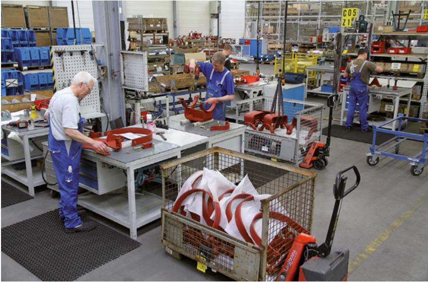
*Pre-assembly of load chains*
