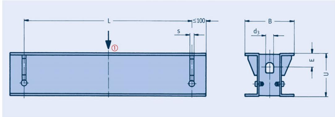
The permissible center load is to be taken from the respective trapeze load group (3<sup>rd</sup> digit or 3<sup>rd</sup> and 4<sup>th</sup> digits in the type designation).
