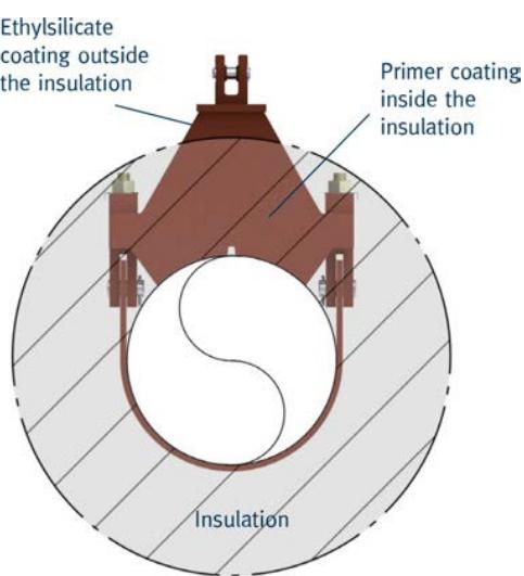
Coating in example of pipe clamps, insulated at T > 350°C
