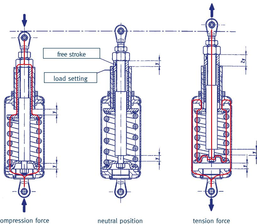
For LISEGA sway braces a free stroke of 0 – 25mm can be set. The travel is reduced in compression and tension directions in accordance with the free stroke selected.
