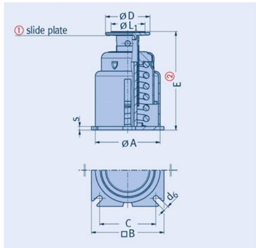
$$E [\text{mm}] = E \text{ at min. load} [\text{mm}] - \frac{\text{adjustment load} [\text{kN}] - \text{min. load} [\text{kN}]}{\text{spring rate} [\text{N/mm}]} \times 1000$$
