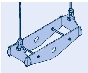
Riser clamp type 48 with connection components
