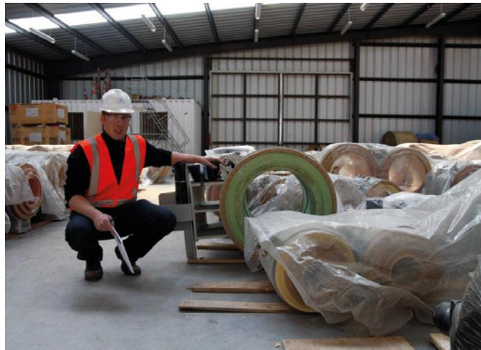
Final inspection of cryogenic clamp bases
