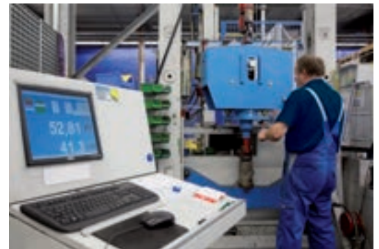
Acceptance testing of a constant hanger
