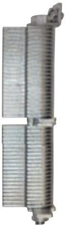
The blocking device for spring hangers and spring supports types 21, 25, 29 and 20 consist of sheet metal lamellas adjustable to any desired load position. Up to 3 blocking devices can be inserted into a spring hanger.
