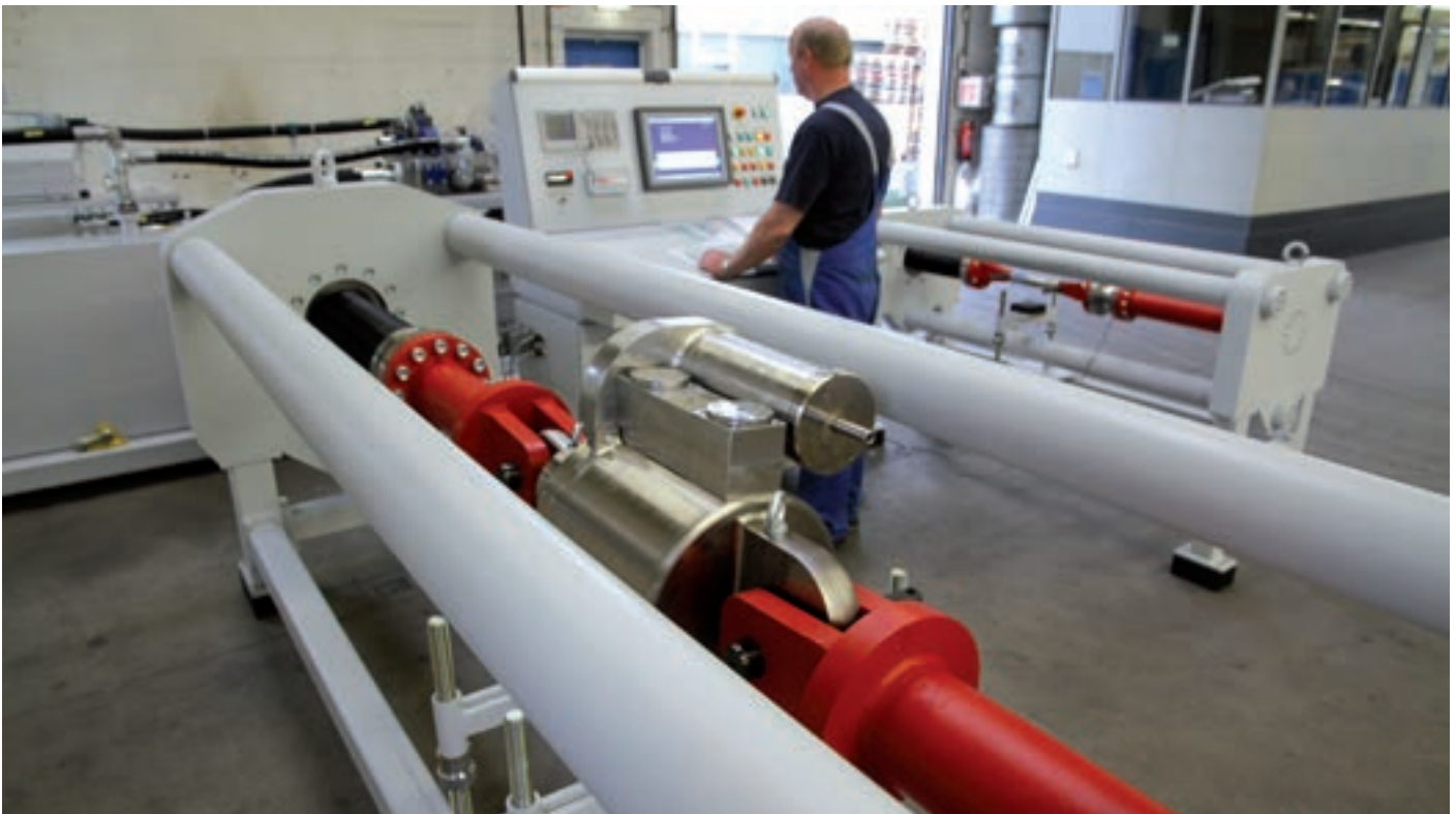
Test bench for snubbers
