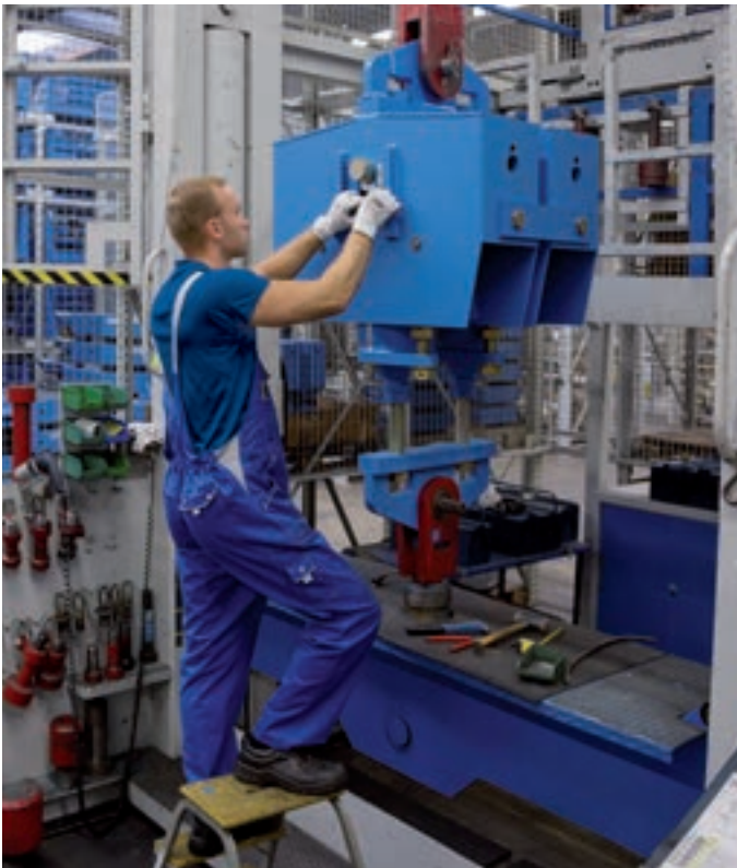
Calibration, testing and blocking of a constant hanger type 12 on a 500kN test bench
