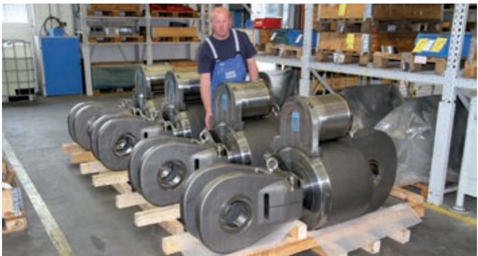
Final inspection of snubbers type 31
