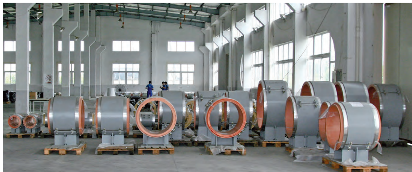
Preassembled insulated pipe supports
