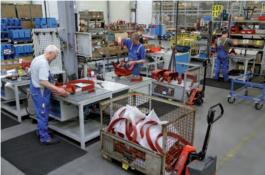
Pre-assembly of load chains
