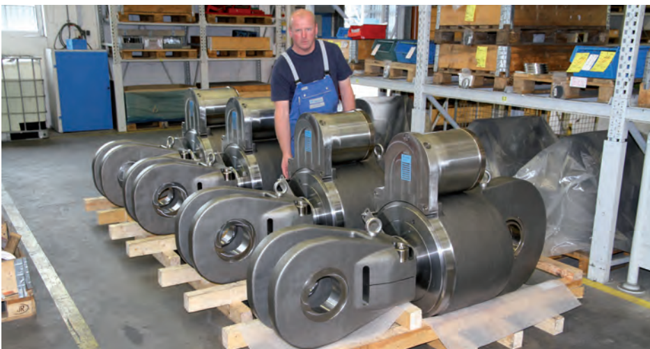
Final inspection of snubbers type 31
