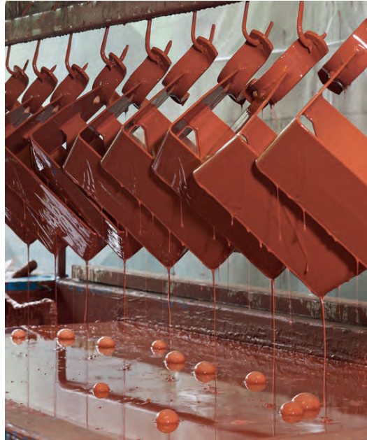
Cataphoretic immersion priming
