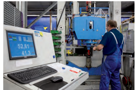
Acceptance testing of a constant hanger
