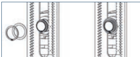
② Assembly of the outer locking ring ③ Completed: deblocked condition
