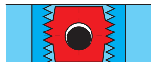
b) Guide pin lies at bottom: Set load of constant hanger is smaller than weight applied. Loosen connecting rod or increase set load.
