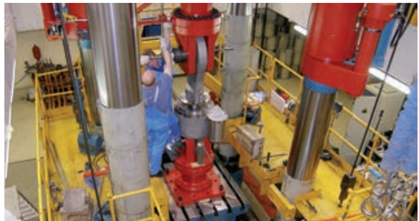
Special testing of snubbers type 31. Test load up to 1,930,000lbs [8600kN]
