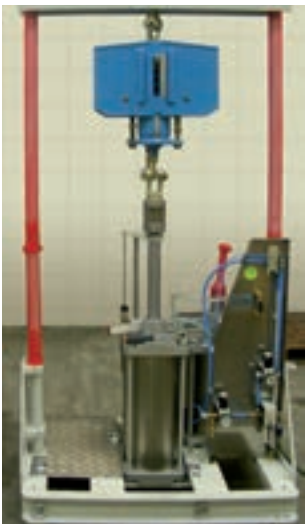
Testing constant hangers on-site with a mobile test bench
