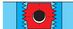
c) Guide pin lies on top: Set load of constant hanger is larger than weight applied. Tighten connecting rod or decrease set load.
