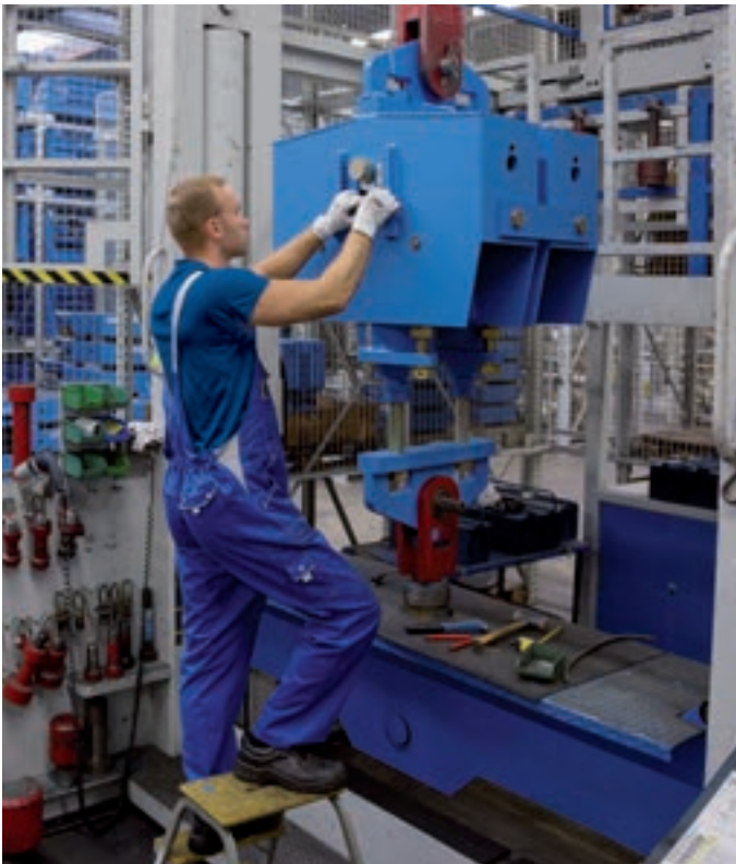
Calibration, testing and blocking of a constant hanger type 12 on a 112405 lbs [500kN] test bench
