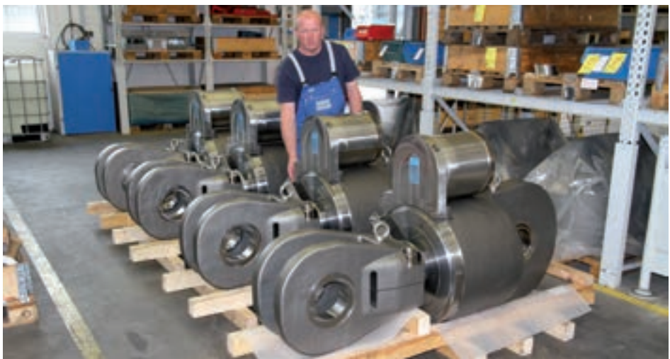
Final inspection of snubbers type 31
