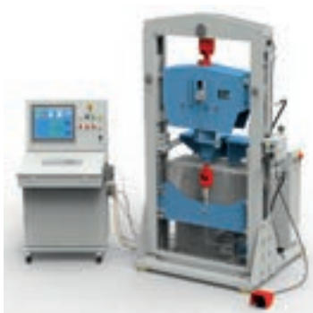
Testing a constant hanger on a LISEGA 26977lbs [120kN] test bench
