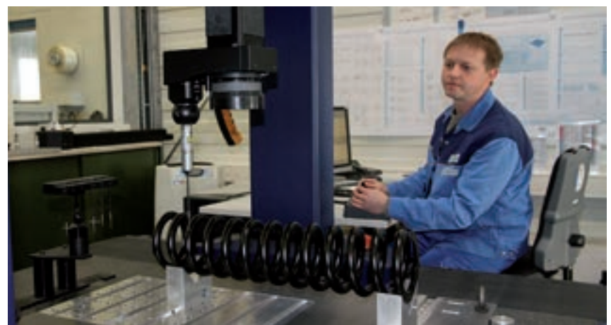
Spring testing at material reception
