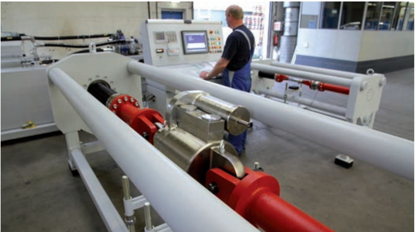
Test bench for snubbers
