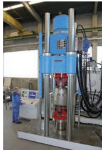
562,000lbs [2500kN] test bench at LISEGA
