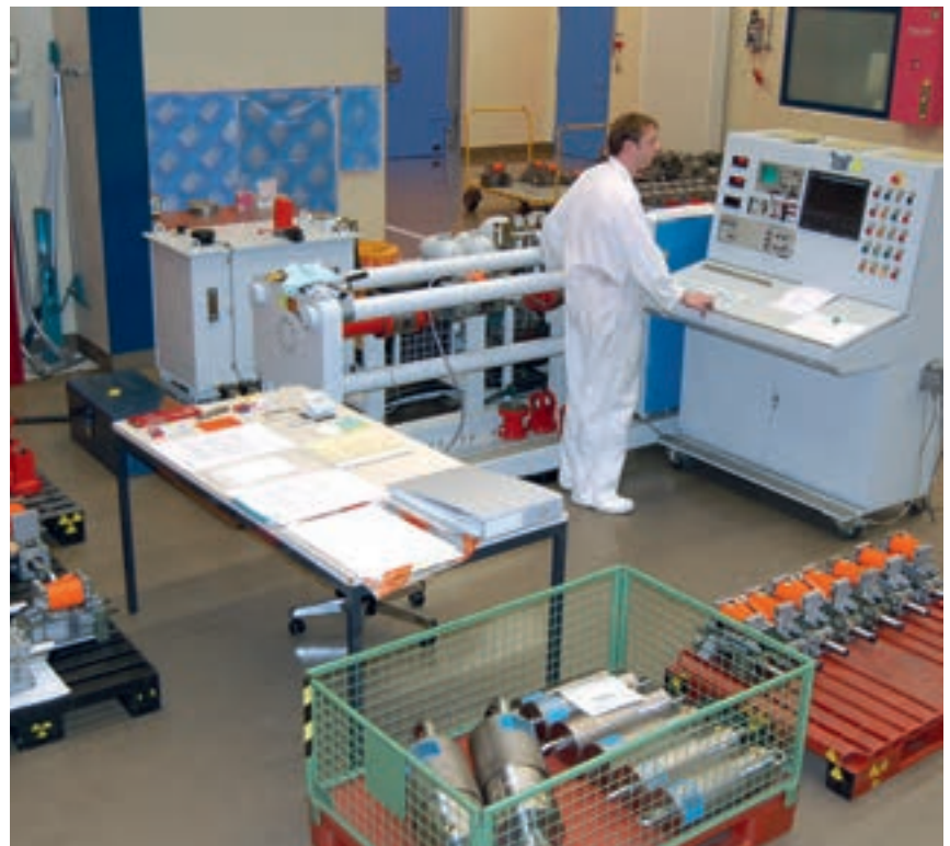
Testing snubbers of different makes at the plant using a mobile LISEGA test bench.
