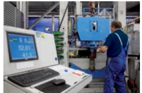
Acceptance testing of a constant hanger
