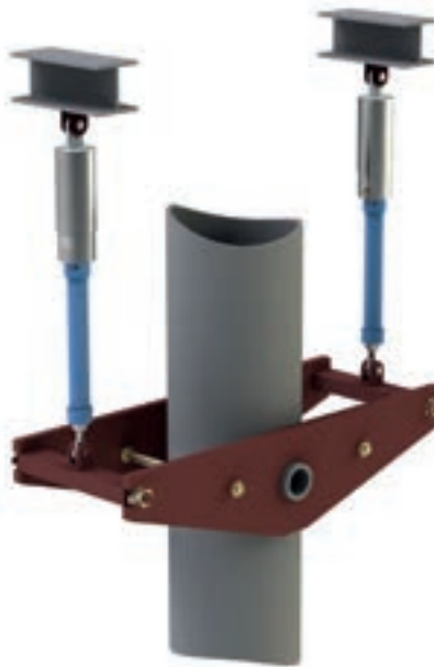
Restraint of a vertical pipe system section by type 30 snubbers with installation extension type 33 and dynamic clamp type 34.
