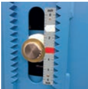
Travel scale with cold/hot marking
