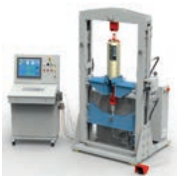
Testing a spring hanger on a LISEGA 26977lbs [120kN] test bench
