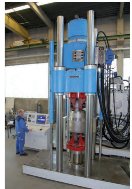
2500kN test bench at LISEGA
