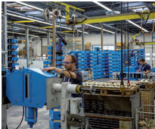
Final assembly of a constant hanger
