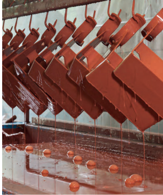
Cathaphoretic immersion priming
