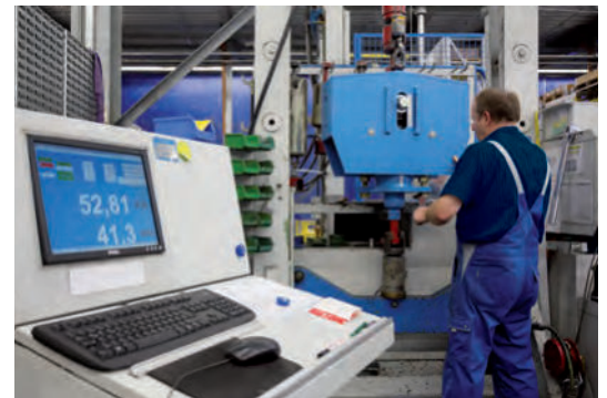
Acceptance testing of a constant hanger
