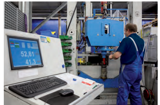
Acceptance testing of a constant hanger
