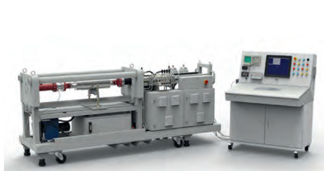
Mobile LISEGA 50kN snubber test bench PR50
