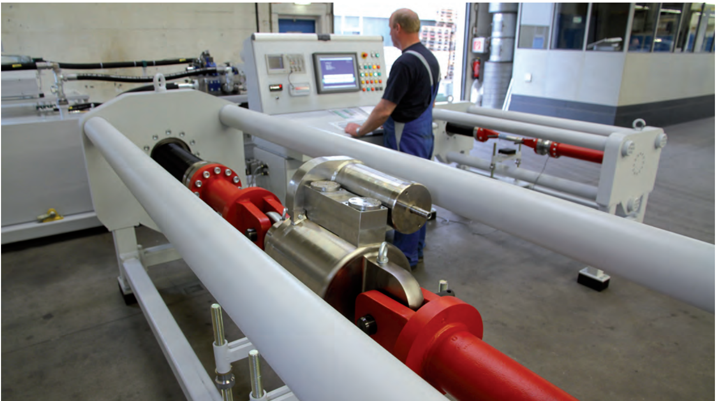
Test bench for snubbers
