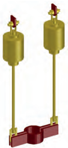
LISEGA standard supports in SmartPlant® 3D
