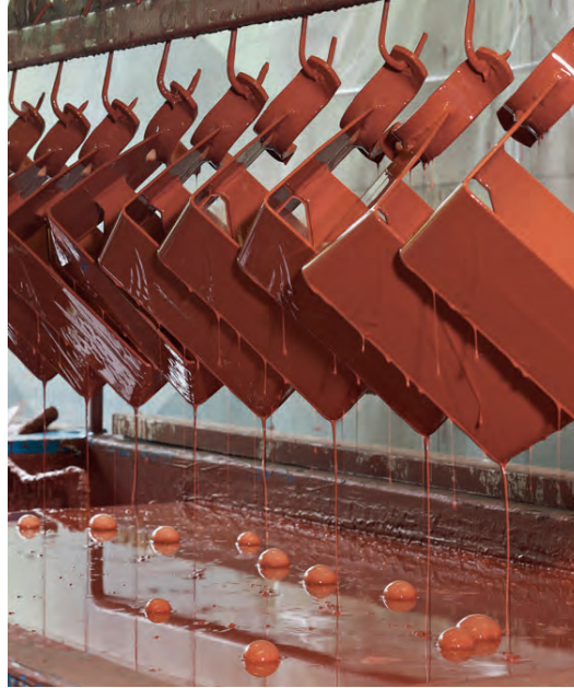
Cathaphoretic immersion priming
