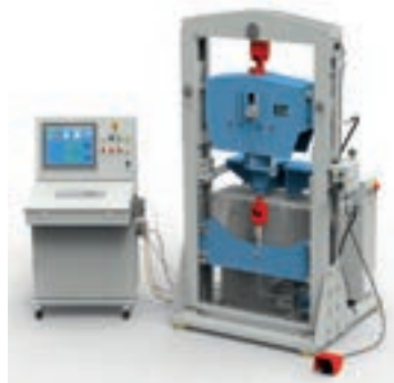
Testing a constant hanger on a LISEGA 26977 lbs [120kN] test bench
