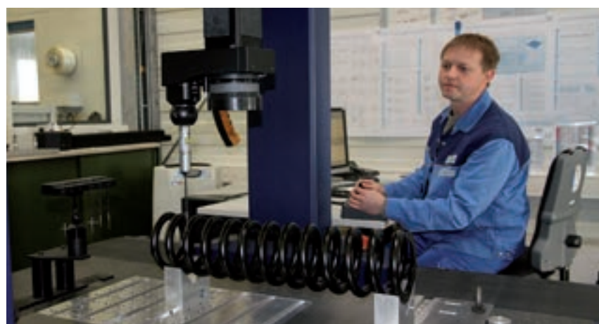
Spring testing at material reception
