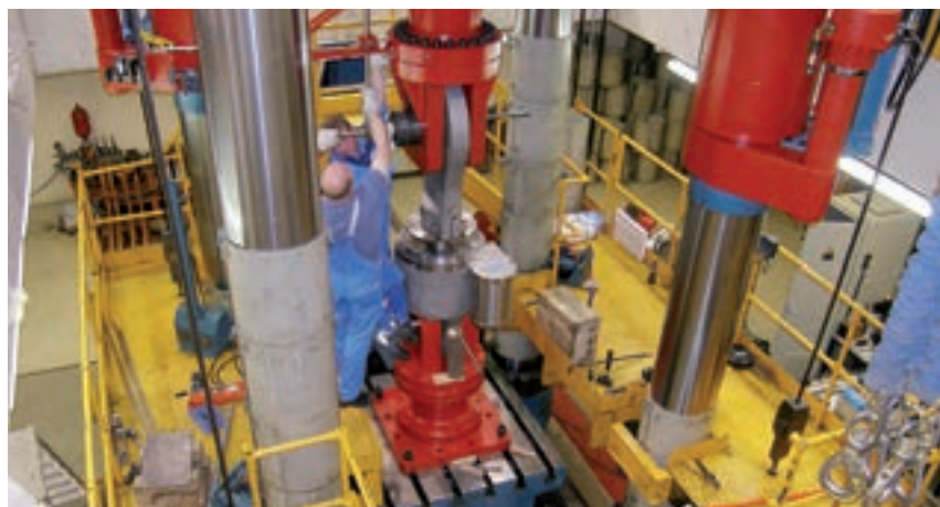
Special testing of snubbers type 31. Test load up to 1,930,000 lbs [8600 kN]
