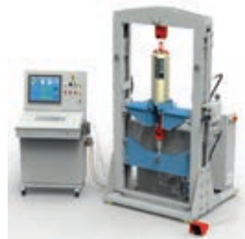
Testing a spring hanger on a LISEGA 26977 lbs [120kN] test bench
