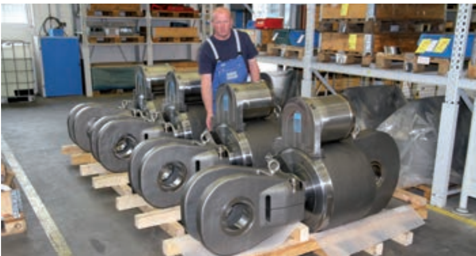
Final inspection of snubbers type 31
