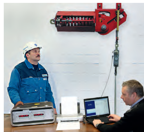
Testing constant hangers on site with mobile test bench
