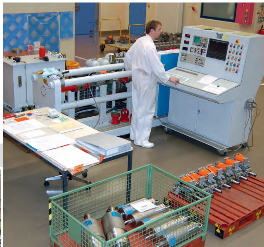
Performance testing of shock absorbers of different makes at the plant with one of LISEGA's mobile test benches
