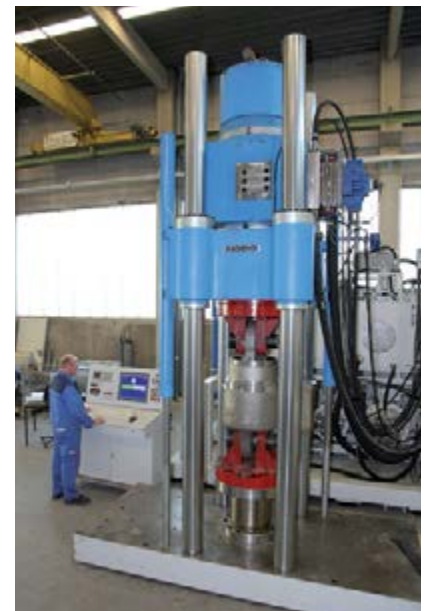
2500kN test bench at LISEGA
