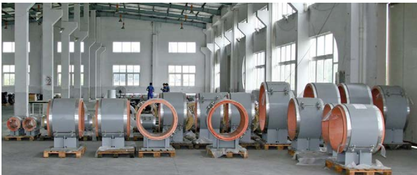
Preassembled insulated pipe supports
