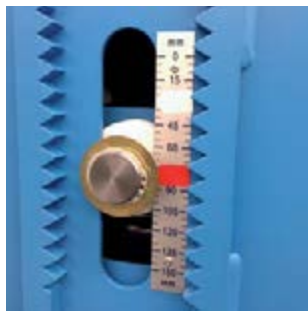
Travel scale with cold/warm marking
