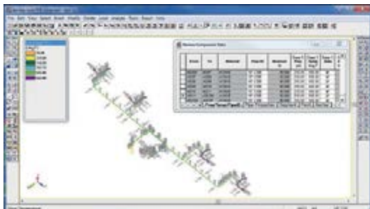
Pipe systems in AutoPIPE®
