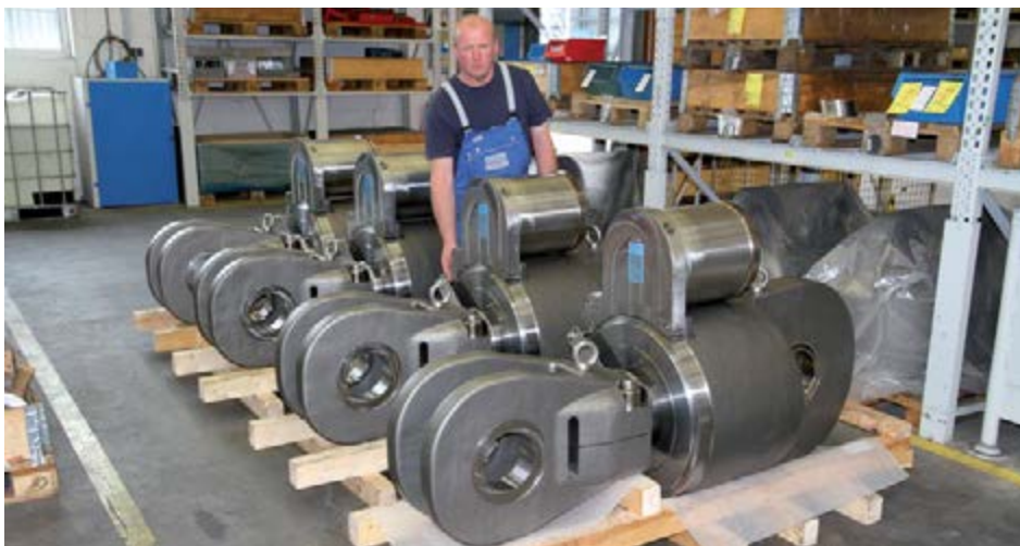
Final inspection of snubbers type 31
