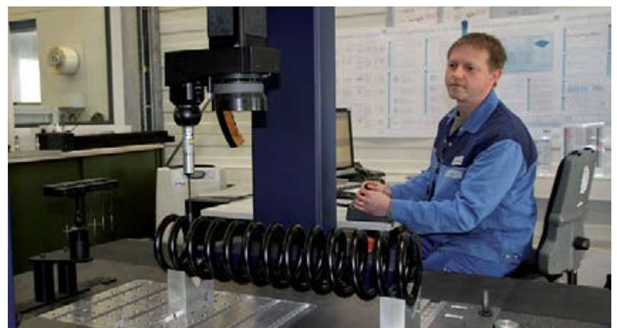
Spring testing at material reception
