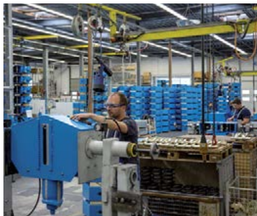
Final assembly of a constant hanger
