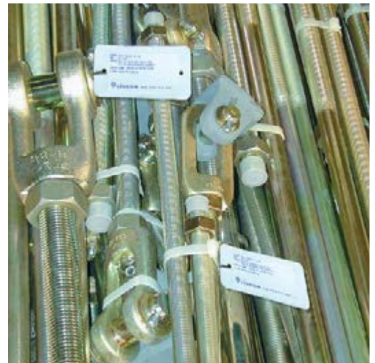
Load chains, pre-assembled, bundled and marked
