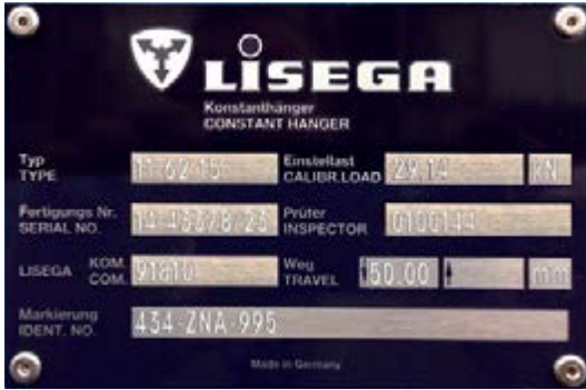
Name plate with stamped operating data
