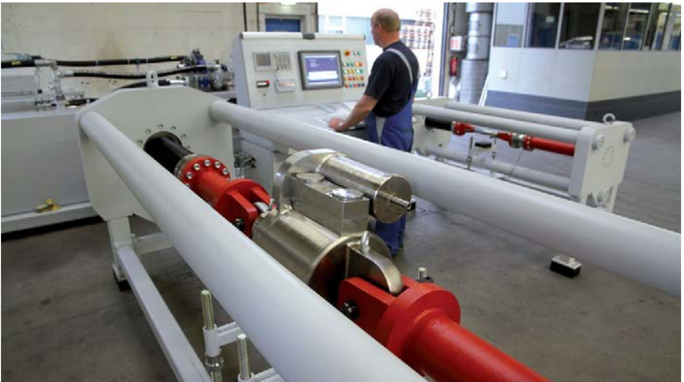
Test bench for snubbers
