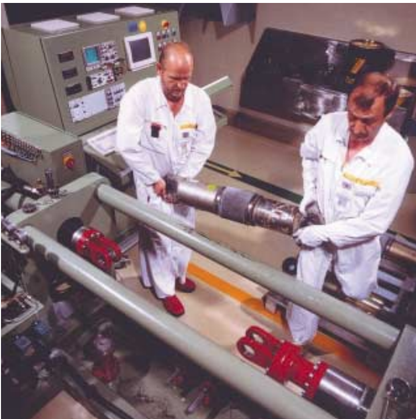
Testing PSA shock absorbers at the plant with a mobile LISEGA test bench.
