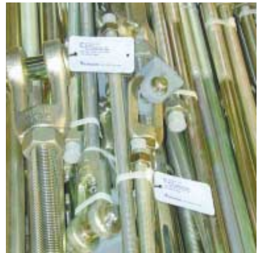
Load chains, preassembled, bundled and marked
