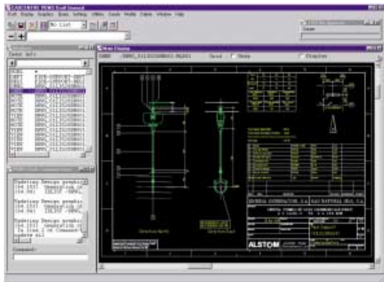
2D support drawing generated directly from PDMS 3D model
